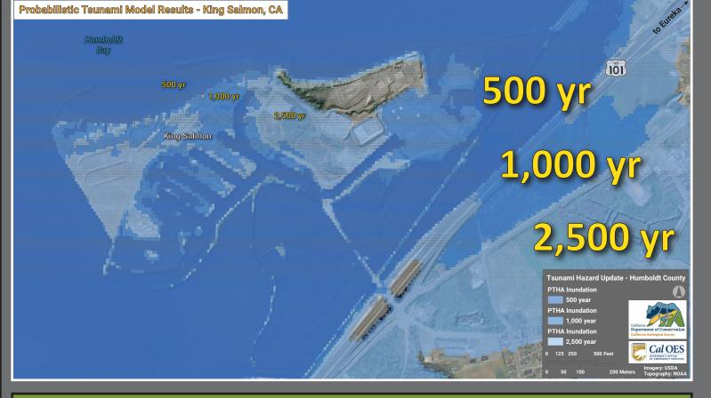
The map above shows the inundation model results for sunami with three rates of recurrence. Note how the sunami with a longer recurrence interval is larger (extends further inland) than the tsunami with a shorter recurrence interval.
