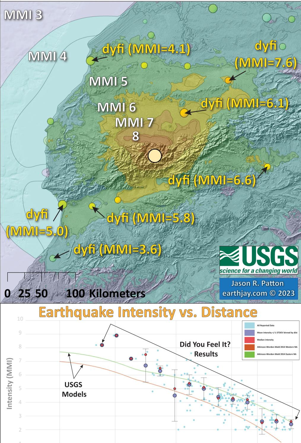
Distance to Earthquake (km) **SHAKING** Not Felt Weak Moderate Strong **Very Strong** Violent Light Severe Extreme Very Heavy **DAMAGE** Note None None Very Light Light Moderate Moderate/Heavy Heavy 0.3 2.76 11.5 74.7 **PGA** (%g) < 0.05 6.2 21.5 40.1 >139 PGV (cm/s) 20 < 0.02 0.13 1.41 4.65 9.64 41.4 85.8 >178 5 **INTENSITY** 1 2-3 4 6 7 9 10 8
