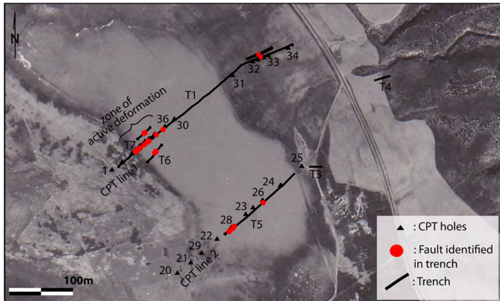
Figure 4. Detailed map of the area of the two CPT lines and trenches. Dots mark the location of each fault strand identified in the trenches. The color version of this figure is available only in the electronic edition.
