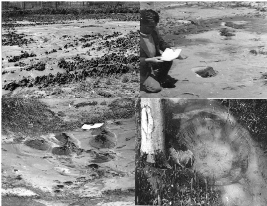
FIG.I.23 - Sand fountains during the earthquake of April 15, 1979.
