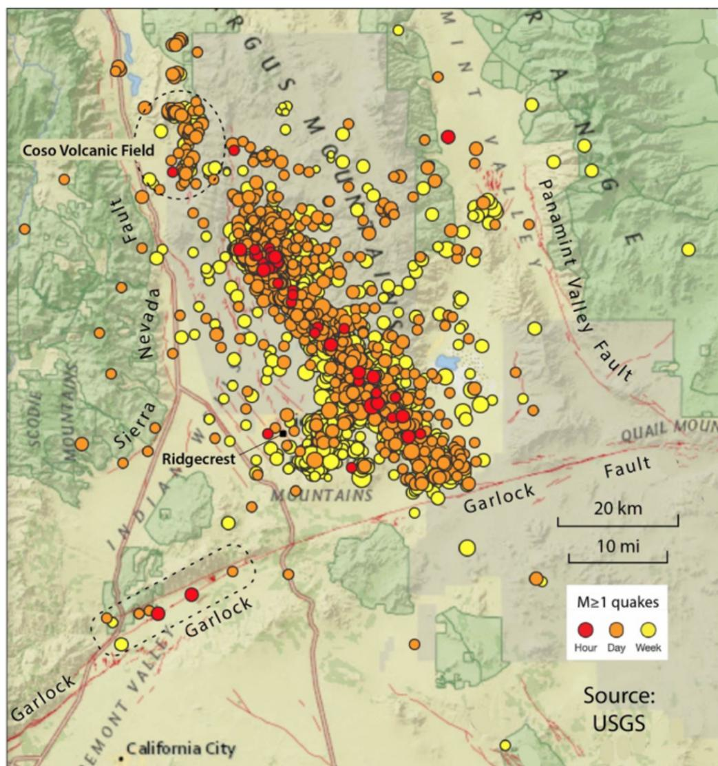
One can see 8-10 small shocks on the Garlock Fault (lower left), and a large cluster at Coso Volcanic Field (upper left).
