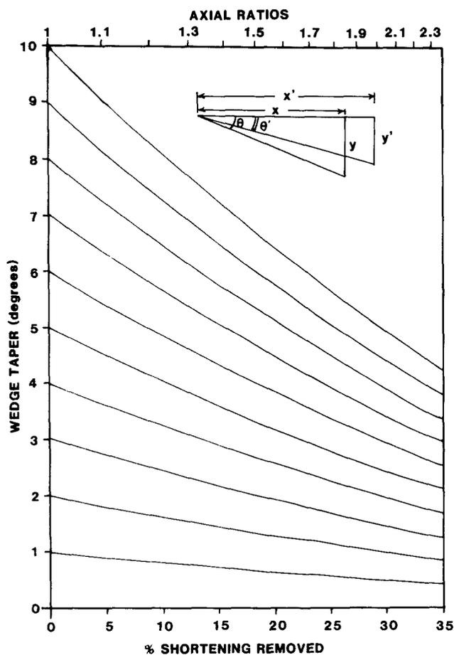
Fig. 17. Change in taper of wedges due to removal of different amounts of strain (see text for details).
