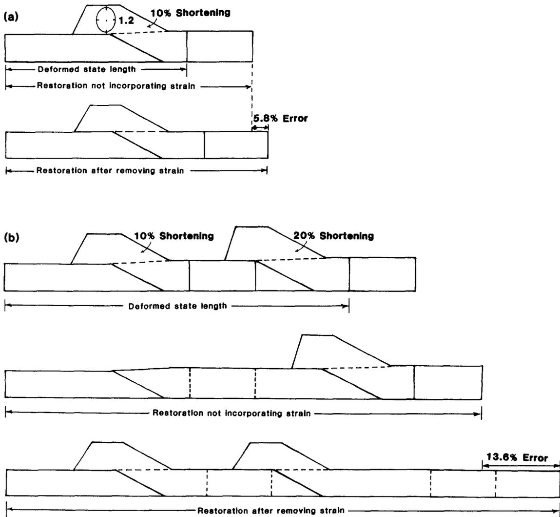
Fig. 14. (a) 10% plane strain internal shortening results in a 5.8% error in line-length balanced equal-area restoration (b) Balancing error is cumulative. Two sheets with 10 and 20% plane strain internal shortening results in 13.6% error at the trailing edge of the second sheet in line-length balanced equal-area restoration.
