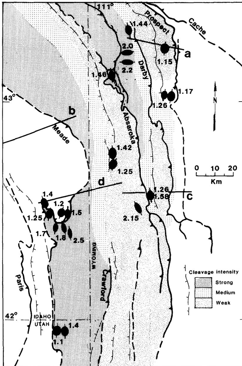
Fig. 10. Map of part of the northern ID-WY FTB showing typical bedding plane strains (YZ) determined from deformed *Pentacrinus* fossils, and from Fry plots on sandstones and oolites. The map also shows intensity of cleavage development in the Twin Creek Formation for parts of the area. Locations of cross-sections (Fig. 9) are shown.
