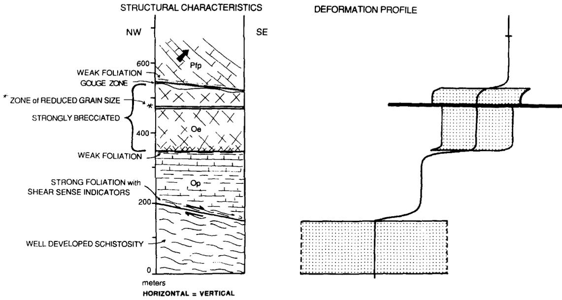
Fig. 5. An example of 'bundled deformation profile' with several weak zones of intense shearing from the Pequop Mountains, Nevada.
