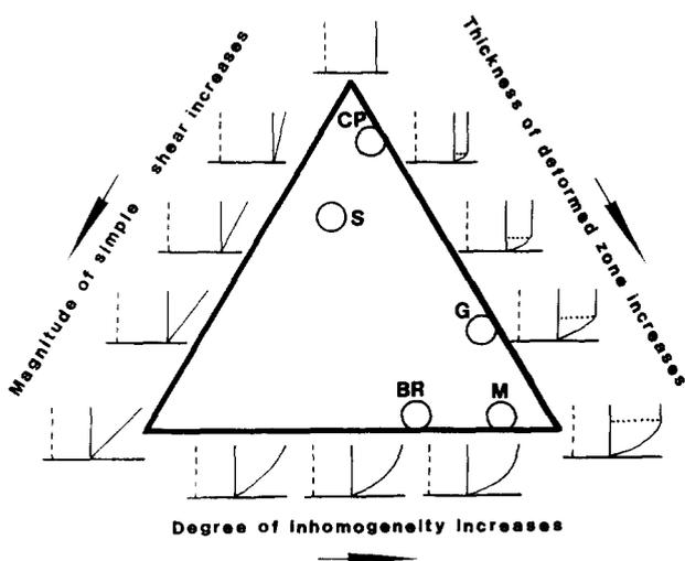
Fig. 4. Triangle diagram showing possible variations in shape of deformation profiles due to variations in magnitude of simple shear, thickness of simple shear zone at base of sheet, and degree of inhomogeneity in sheet movement. Deformation profiles from Fig. 6 are roughly plotted to show range of variations seen in natural examples: Cumberland Plateau (CP), Glarus (G), Särvi (S), Morcles (M) and Blue Ridge (BR) thrust sheets.
