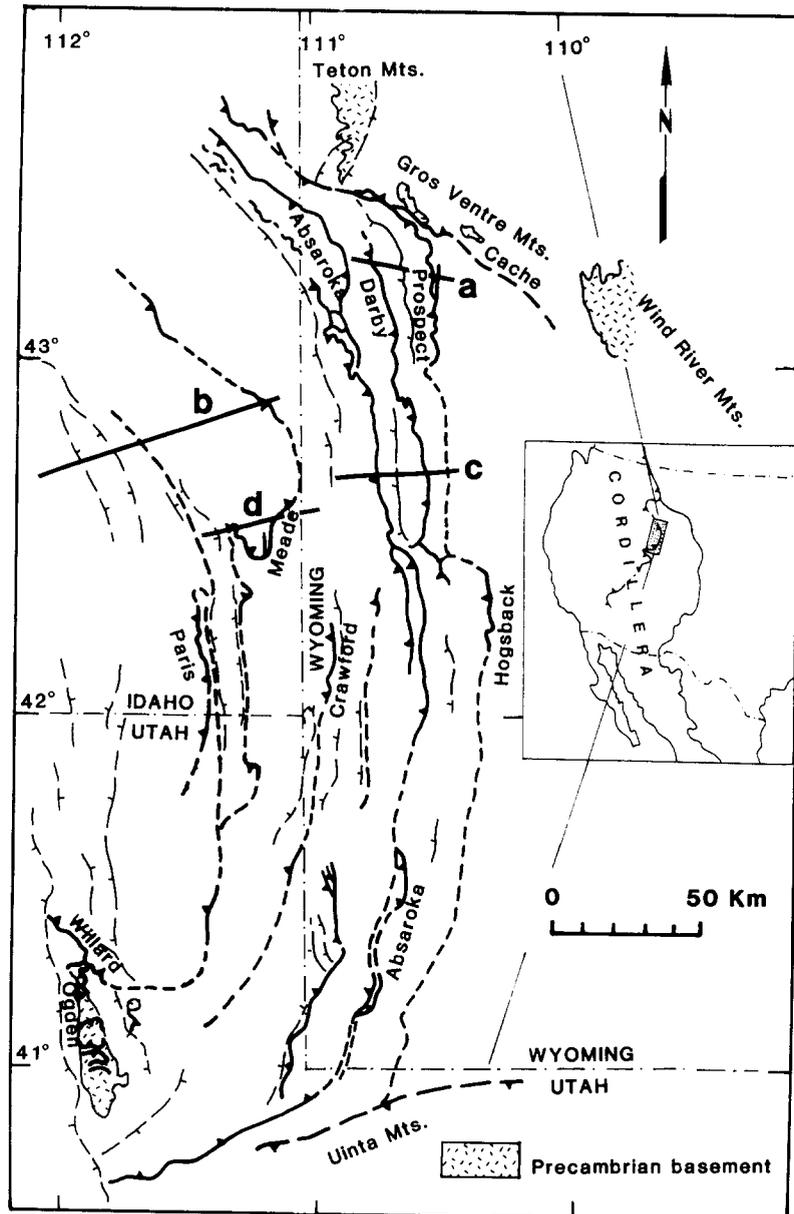
Fig. 7. Tectonic map of Idaho-Utah-Wyoming fold-and-thrust belt showing the main thrust faults and listric normal faults (after Coogan & Royse 1990). Locations of cross-sections (Figs. 9a-d) are shown.
