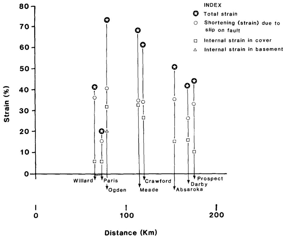
Fig. 12. Variations in internal strain, strain due to slip on major faults, and total strain (all expressed as % shortening) in the main thrust sheets of the ID-UT-WY FTB. Note the dramatic drop in internal strain in the Willard and Paris thrust sheets.
