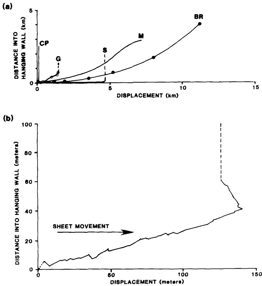
Fig. 6. (a) Deformation profiles of the Cumberland Plateau (CP), Glarus (G), Särvi (S), Morcles (M) and Blue Ridge (BR) sheets compared at the same scale. Note the general pattern of increasing thickness of basal shear zone from foreland to hinterland. (b) Composite deformation profile of the Cumberland Plateau thrust sheet, Southern Appalachians (after Wojtal, 1982). The basal shear zone extends ~60 m into the hanging wall.
