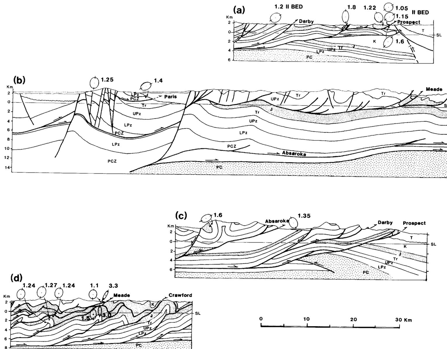
Fig. 9. Cross-sections of parts of the ID-WY FTB showing typical  $XZ$  strain ratios determined from Fry plots on oolites and sandstones. Locations of cross-sections are shown on Figs. 7 and 10. (a) Strain variation in frontal part of the Prospect thrust sheet. (b) Strains within the Paris sheet in SE Idaho. (c) Strains in the Absaroka and Darby sheets, southeast of Star Valley, Wyoming. (d) Strains in the Meade sheet and the Sheep Creek slice of the Crawford system.
