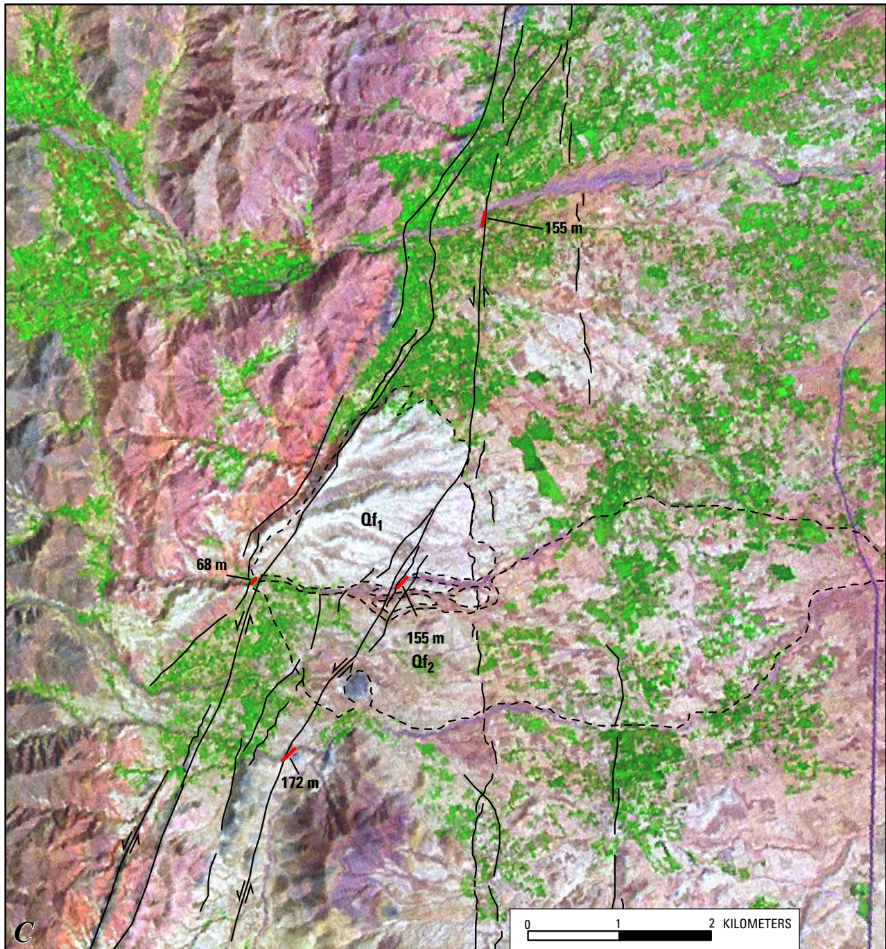
Figure 6C. Mapped strands on the Paghman fault (pl. 1, no. 59) northwest of Kabul. Black lines are mapped fault strands on Quaternary alluvium and bedrock; arrows show directions of movement on fault strands. The fault zone contains multiple strands that offset stream channels varying amounts. Measurements, in meters, show where major streams have been left-laterally displaced by faults. Red solid lines show selected measurements. The large, white, old alluvial fan ( Qf_1 ), has been transported northward along the fault relative to its original source drainage, and a new, younger fan ( Qf_2 ) is being deposited in its previous position. Image is a panchromatically enhanced Landsat image that merges bands 7+4+1. See figure 6 for location.
