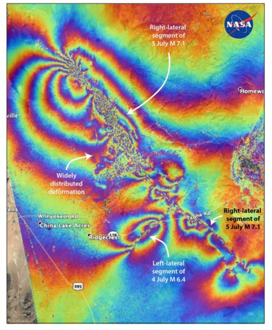
The interferogram is derived from the ALOS-2 satellite, operated by the Japan Aerospace Exploration Agency (JAXA), with images taken before (16 April 2018) and after (8 July 2019) the earthquakes. Each color cycle represents 11.45 cm (4.5 inches) of ground displacement in the radar line-of-sight (28° from vertical and roughly east).
