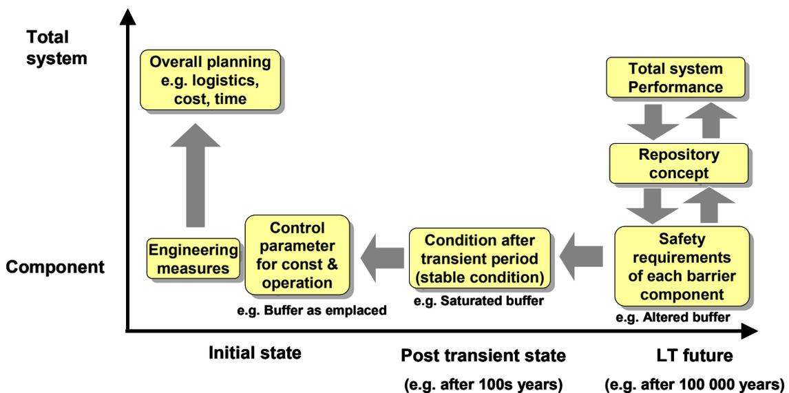
**Figure A.2 Illustration of how long-term safety requirements influence the engineering measures employed and the overall planning of repository construction and operation.**
