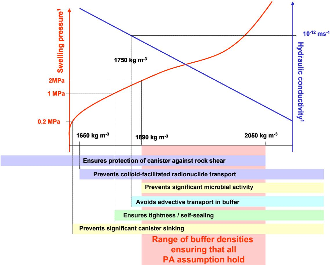
**Figure A.5** Deriving a range of buffer density that, if maintained, should ensure that all the safety functions of the buffer are provided (typical PA assumptions hold).
