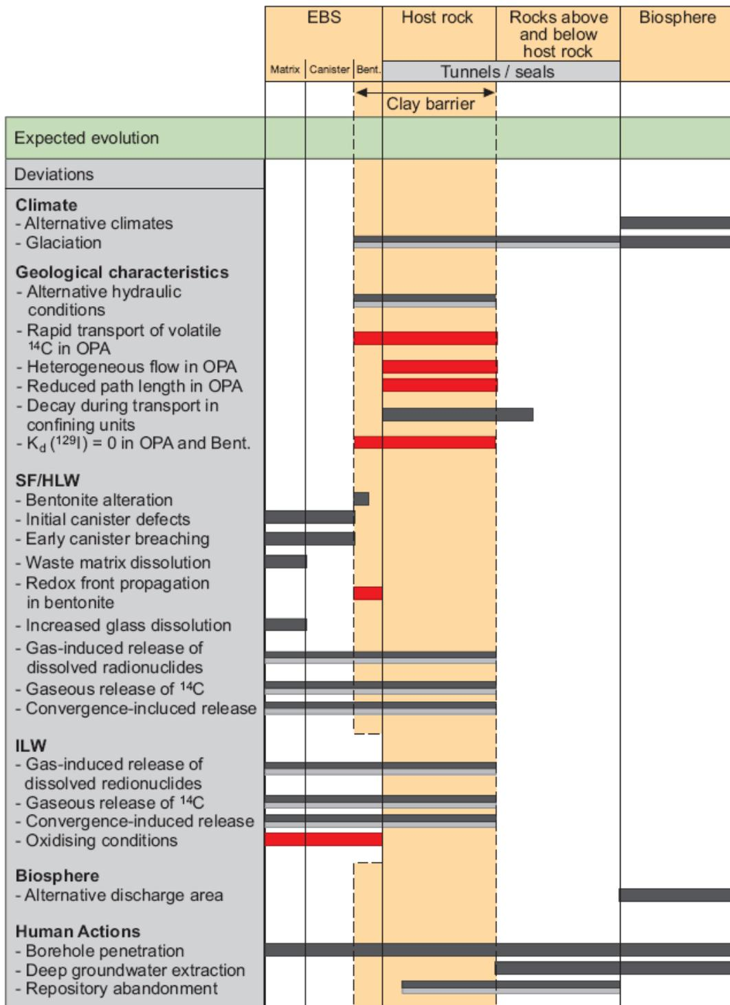
Figure 3.5 Range of influence of possible deviations from the expected evolution of the Project Opalinus Clay disposal system (after Figure 5.7-1 in Nagra, 2002a).
