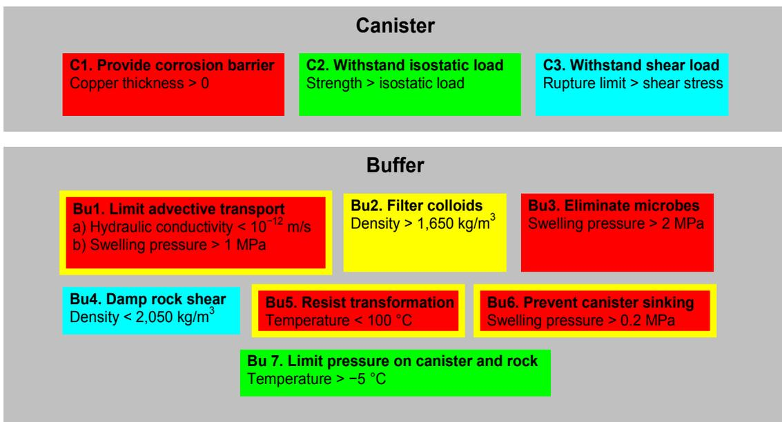
Figure 3.6 Safety function indicators and criteria for the SR-Can canister and buffer (after SKB, 2006).
