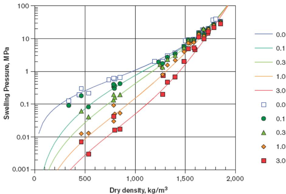
**Figure A.4 Relationship between buffer swelling pressure, dry density and ionic strength, expressed as molar NaCl concentrations (after Figure 4-7 in SKB, 2006).**
