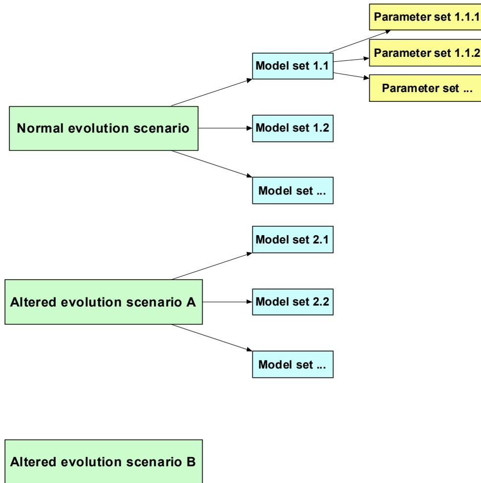
**Figure 3.4 Schematic illustration of the structuring of assessment cases, with each case consisting of a scenario, a model set and a parameter set.**
