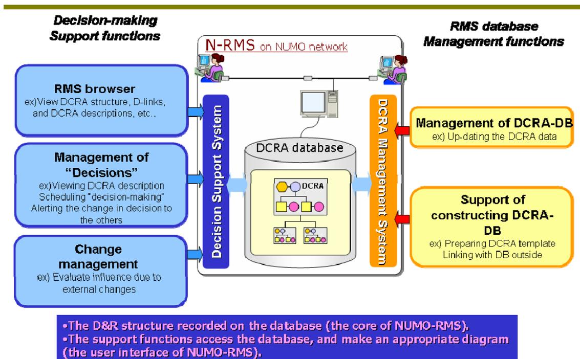
**Figure 4.9 Overall system concept of the N-RMS with two functions – decision-making support function and RMS database management function.**
