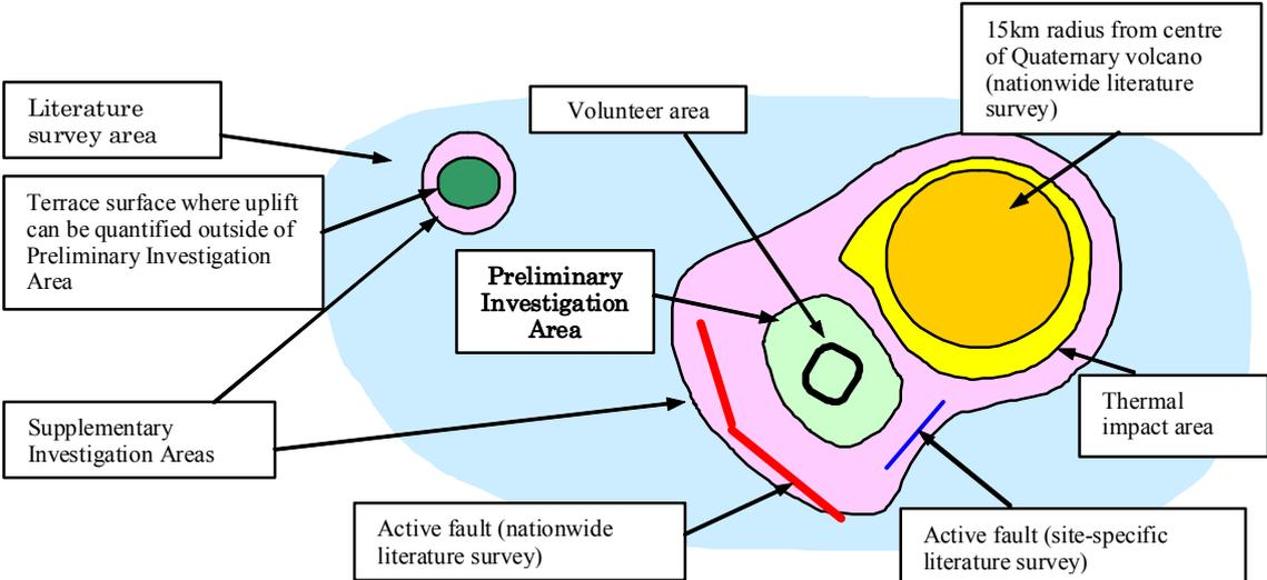
**Figure 2.4 Schematic illustration showing how the legally defined Evaluation Factors for Qualification affect the identification of the location and geometry of a Preliminary Investigation Area (after NUMO, 2004b).**
