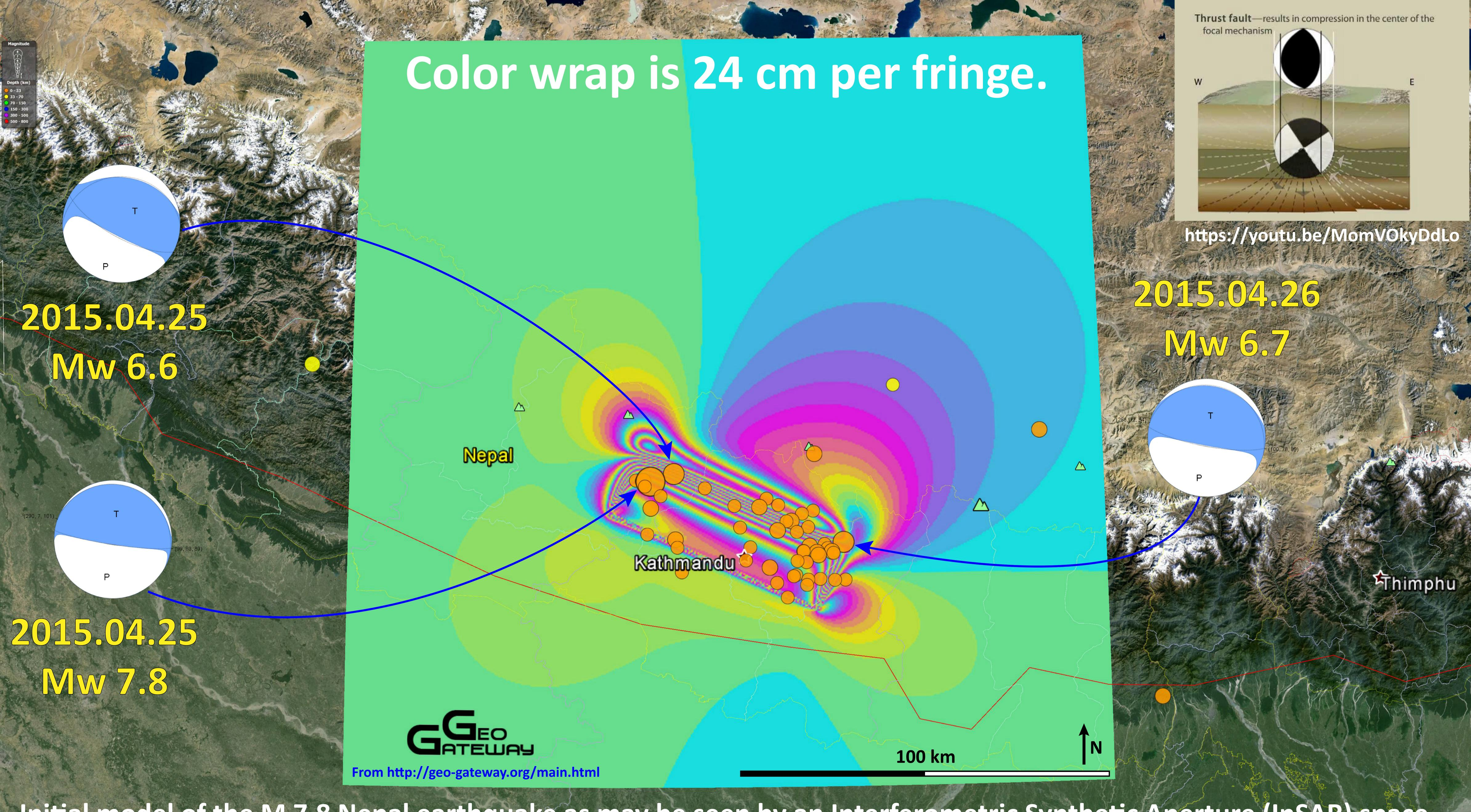
Initial model of the M 7.8 Nepal earthquake as may be seen by an Interferometric Synthetic Aperture (InSAR) space-craft such as Sentinal-1 or ALOS-2 and GPS. The model is based on USGS mechanism of a near horizontal fault and the location of aftershocks. This image shows a synthetic interferogram for a descending pass of –168°, 24 cm wavelength, elevation of 40°. Fault is 11° dip striking 295°. Maximum displacement vector is about 2.3 m.
